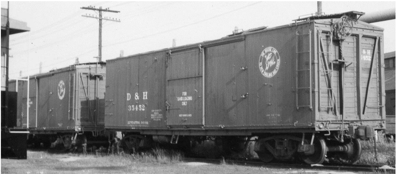
Two D&H shorties downgraded to company sand service. These 14907-built boxcars have both been rebuilt with Indestructible ends, and car 35452 has a power hand brake (but retains her K brakes)
