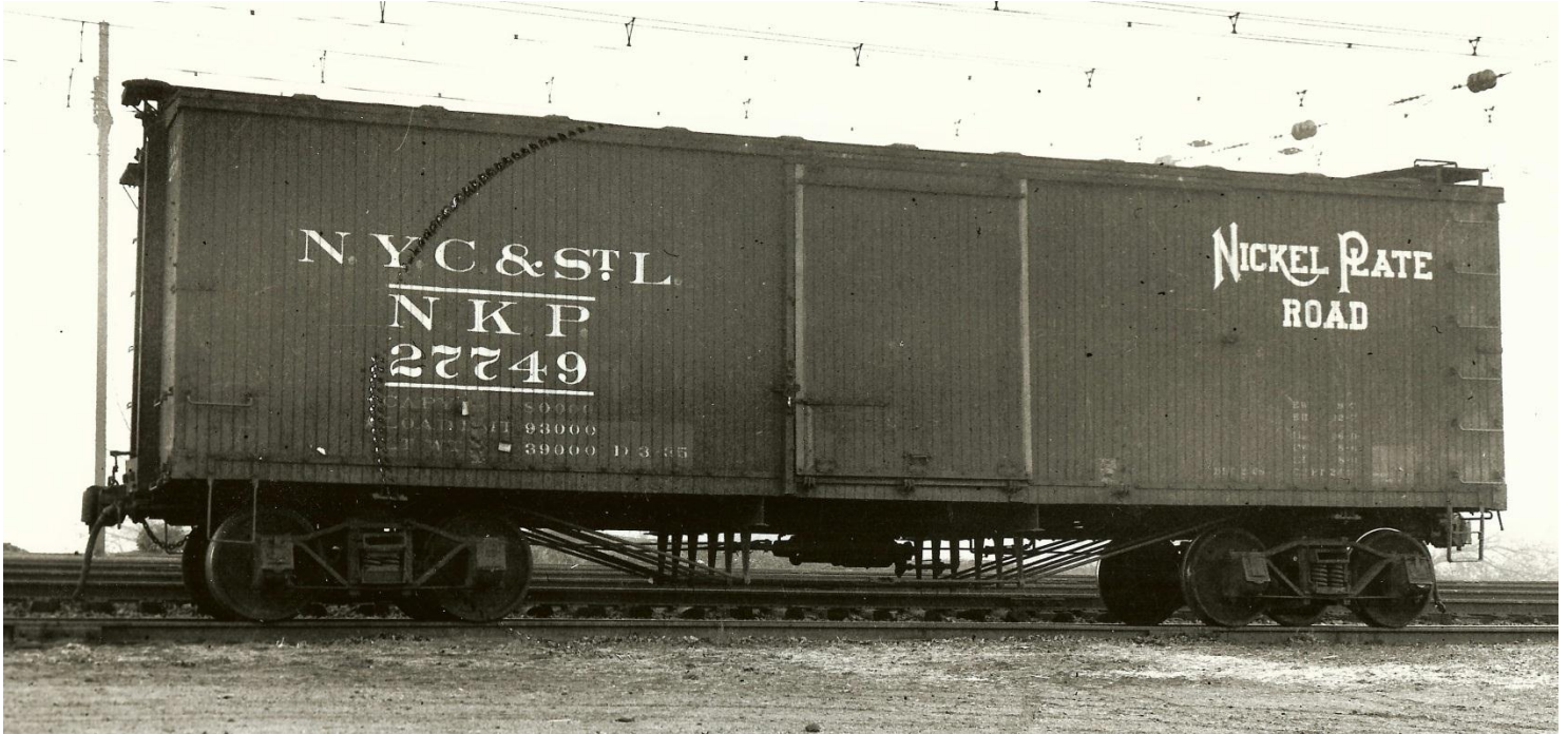
NKP 27749 sits on the New Haven in 1936. Notice that the needle beams (the bars that hold the queenposts in place) are actually steel I-beams, a quick and easy way to tell that an old boxcar has a new steel underframe.
