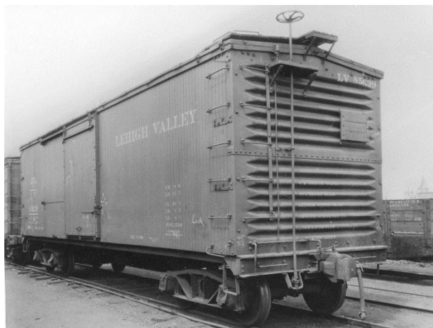
A rebuilt LV 85639 sits around in Long Island in early 1933. Note that the car, although rebuilt with many new all-steel body elements, retains its original archbar trucks.
