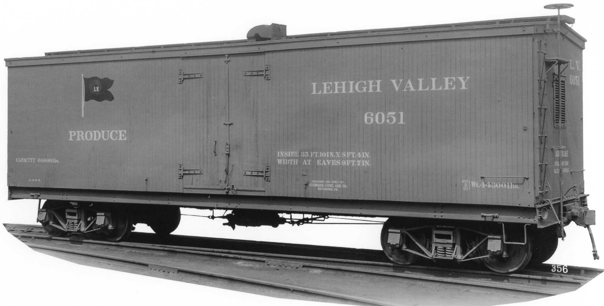
LV 6051 built in 1907 by Standard Steel Car Company as a Produce Car
