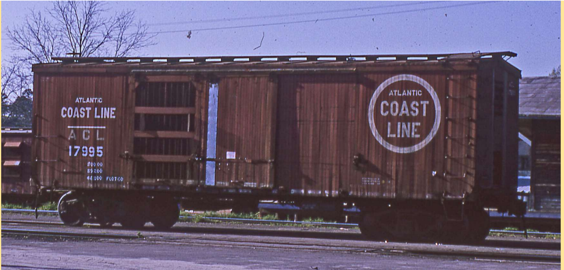
Ron Christensen captured ACL 17995 at Thomasville, Georgia in May 1964. This O-17 class car has a 36-foot interior length and was built in the ACL shops in 1922-23.
